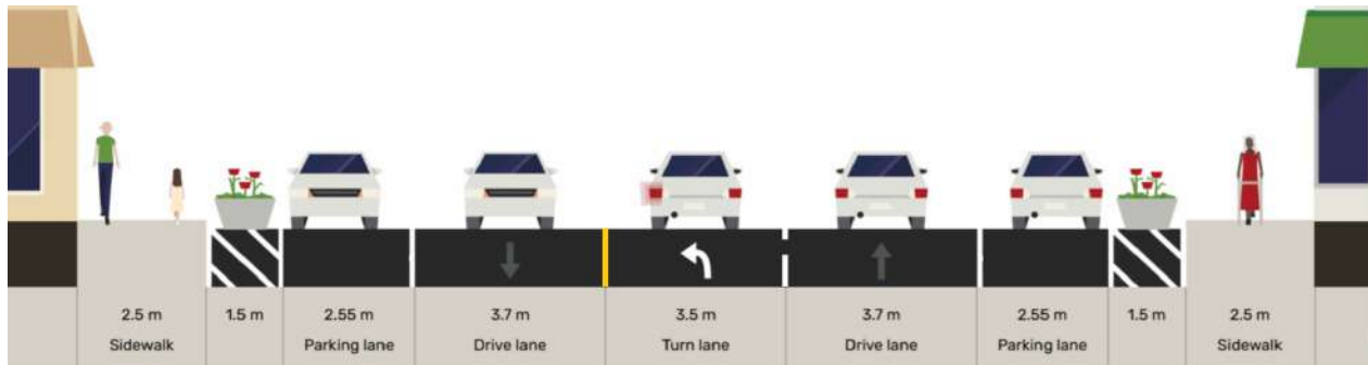
Figure 6.13: Proposed 50 Avenue Downtown Mid-Block Cross-Section C
