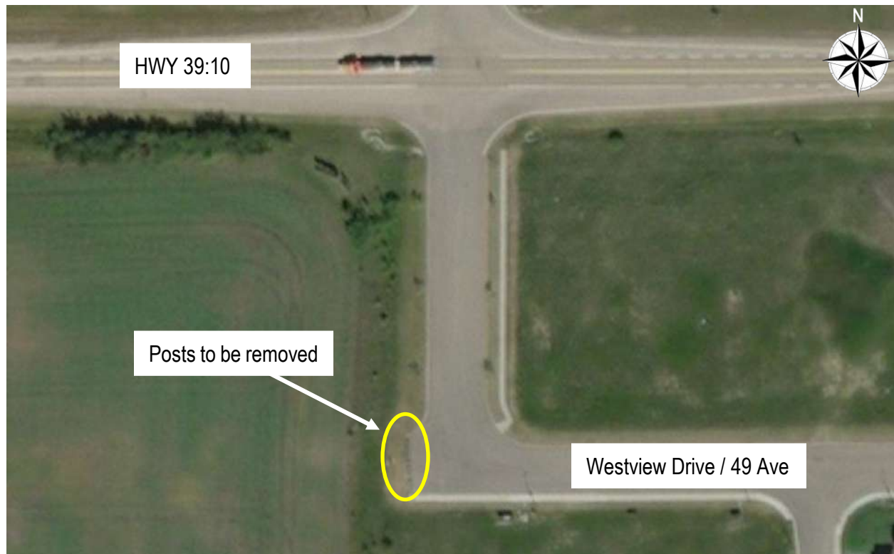
Figure 26 - 49 Ave / Westview Drive Post Removal
